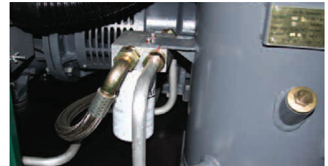
Lubricant filter assembly features a spin-on, full-flow, 12μ, high-efficiency components
